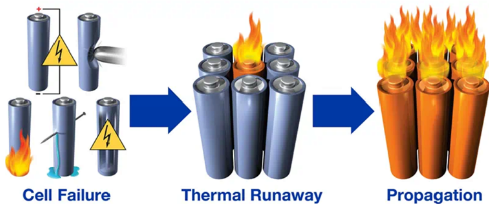
Figure 2: Thermal Runaway and Propagation
